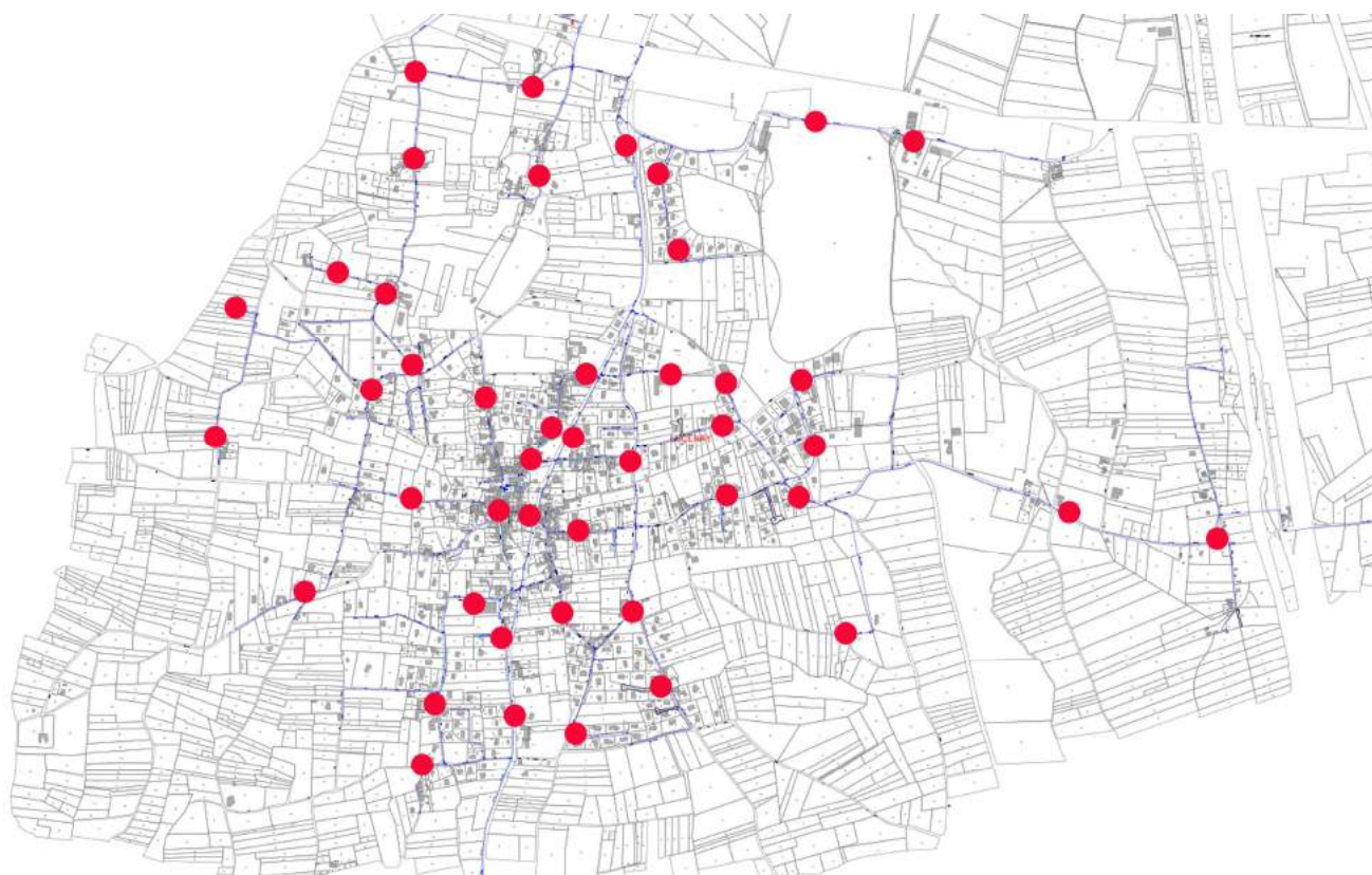
Figure 37 : Situation des poteaux incendie.
