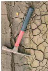
Figure 1.2. Cracks in a soil sample during drying.
