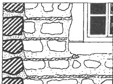
Joints "creusois" dits "à la fourchette"
